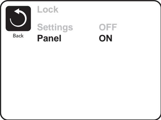
An Unlock Sequence using the navigation buttons can be used from the Lock Screen. The Unlock Sequence is the same for both Panel Lock and Settings Lock.
